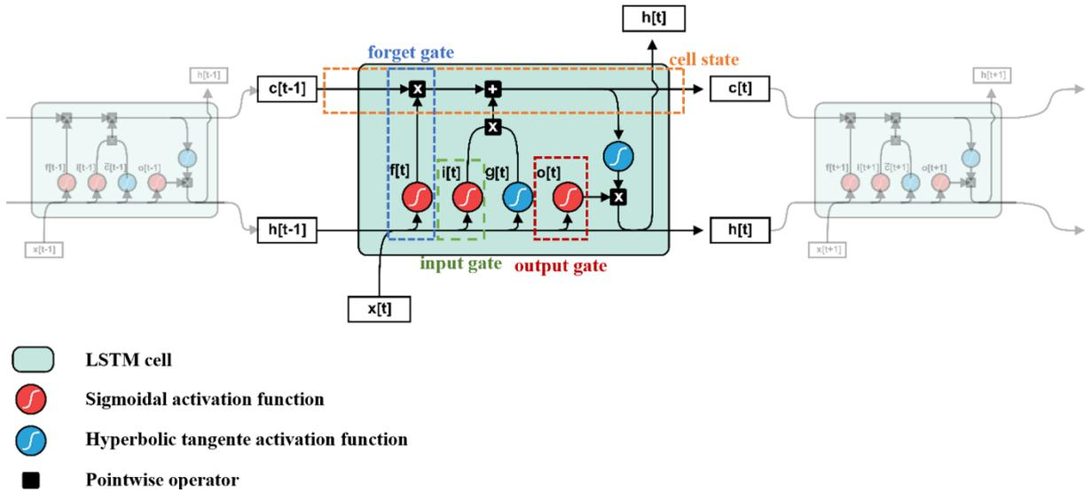
**Figure 4. Long Short-Term Memory cell structure used to simulate and project the river basin's streamflow.**
