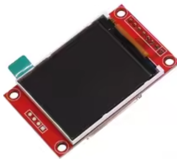
Figura 3.13 – Display TFT 1.8" (driver ST7735).
