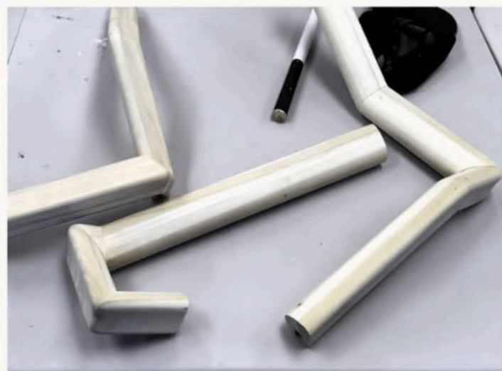
TRANSITIONS MOCKED UP TO TEST FOR COMFORT
