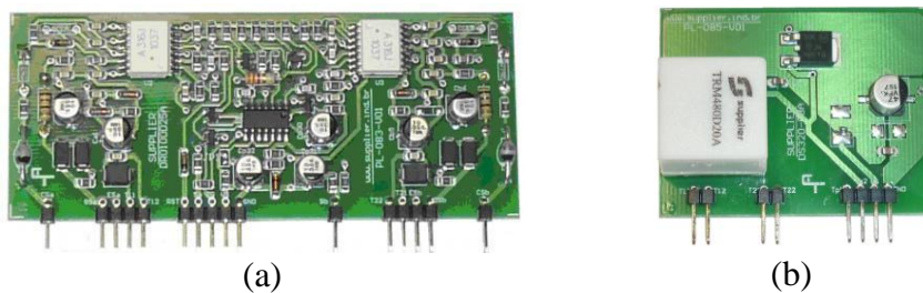
Figura 4.3 - Gatedriver . (a) Drive DRO100D25A; (b) Fonte DS320-08A.
