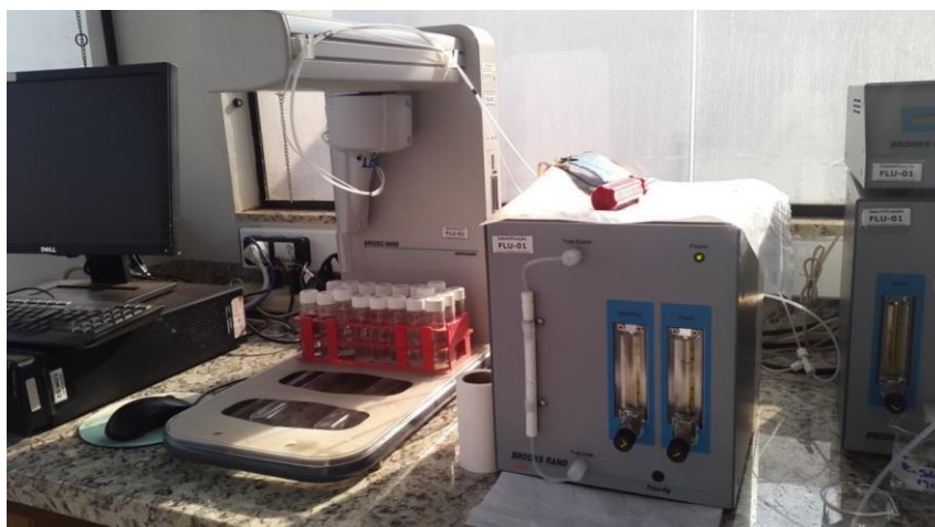
Figura 12: Espectrômetro de fluorescência atômica (AFS) - MERX total mercury and methylmercury analyzer systems.
