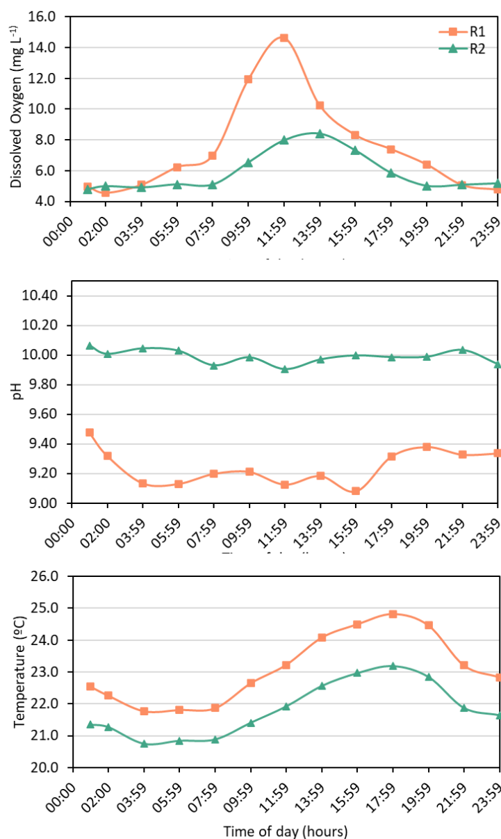
Figure 4-2 - Daily variation of dissolved oxygen, pH, and temperature in reactors with continuous mixing (R1) and intermittent mixing (R2).
