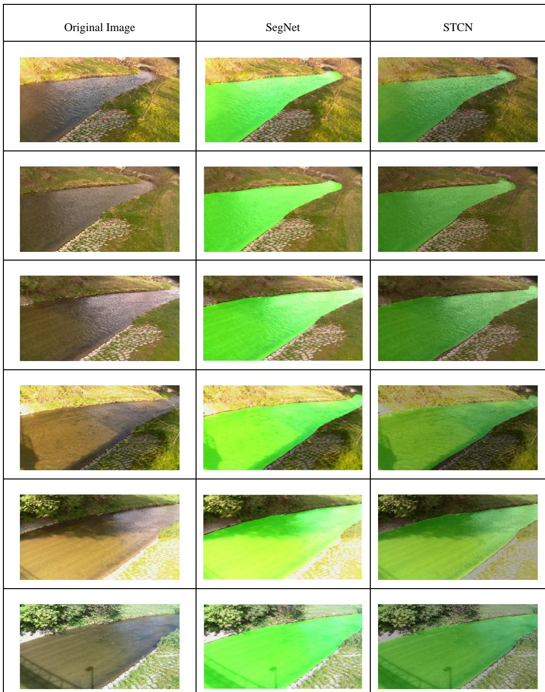
Figure 7. Comparing segmentation between SegNet and STCN.
