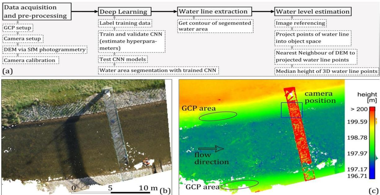
Figure 1. (a) Workflow to automatically extract the water stage from images. (b) Orthophoto and (c) DEM of the area of interest, including an indication of the camera position and ground control points (GCPs) locations.
