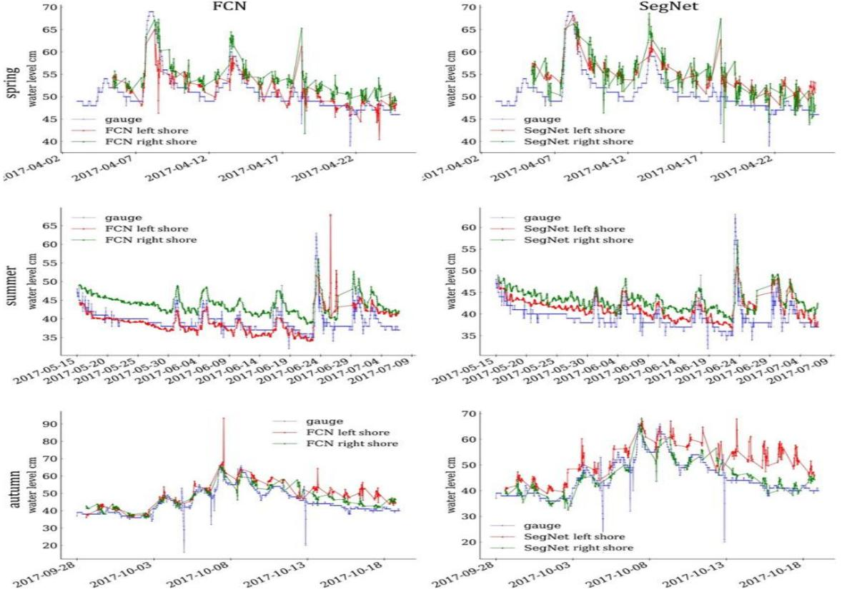
Figure 8. Time series of water stage detection with FCN and SegNet at left and right shore compared to gauge.
